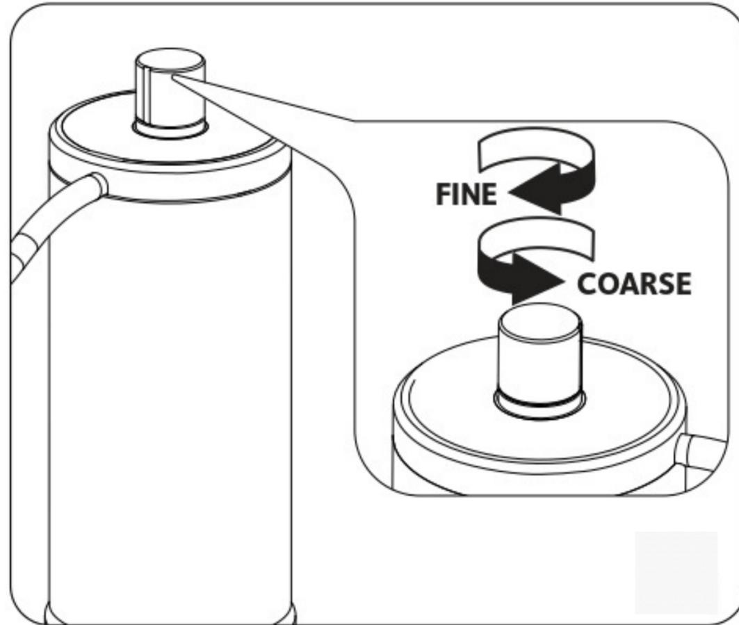
Adjustment of the burrs distance from the top, thanks to the Eureka Micrometric Regulation System (stepped).
